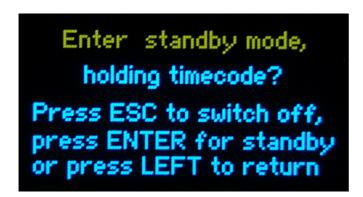
Press ESC for 3 seconds. Standby window will show Press ESC to switch off in 3 seconds Press ENT to enter Standby
